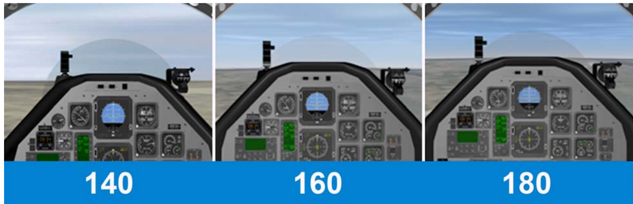
Figure 4.4. Constant Airspeed Climb Pitch Attitudes.
