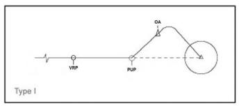
This can be seen in the picture below. In both cases you will get a certain offset from the target, which will give you the correct distance for the final turn and your bombing run. This distance will also give you a chance to find the target by looking to the side. This can be done before turning towards the target and makes it a lot easier.
