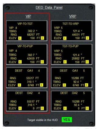
of the tadpole on the HUD you will able to get to the correct approach path faster and easier. This is the whole objective of this setup. Even if you loose all the HUD points, you can still fly this by leaving the IP with the planned track. As you get to the planned distance from the IP, just do the pop-up as planned.
