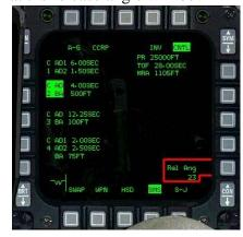
can select the functions for the Arming Delay and the Burst Altitude, but at this time we want to change the Release Angle. You can find this on the lower right bottom of the screen. Again you can see that 23deg has been set and by pushing the button MFD10 to the right of the text, you will go to
