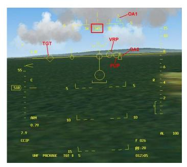
the OA2. At this time I just start a slow turn to the right and fly over the VRP to the PUP. How much before the VRP you start the turn to the PUP depends on your speed, the angle and the amount of G you will use. After passing the VRP the important thing to do now is to fly to the PUP with the planned Pull Heading. Make some small error corrections, but don't make large turns.
